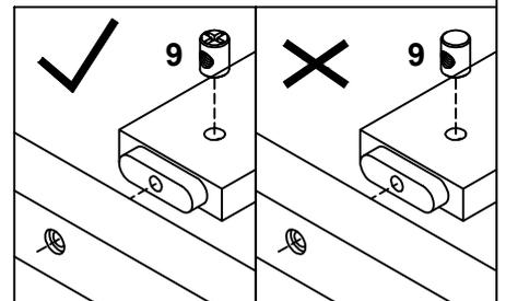
Note: Part 9 will face up with the "x" mark on it, otherwise it cannot be tightened
