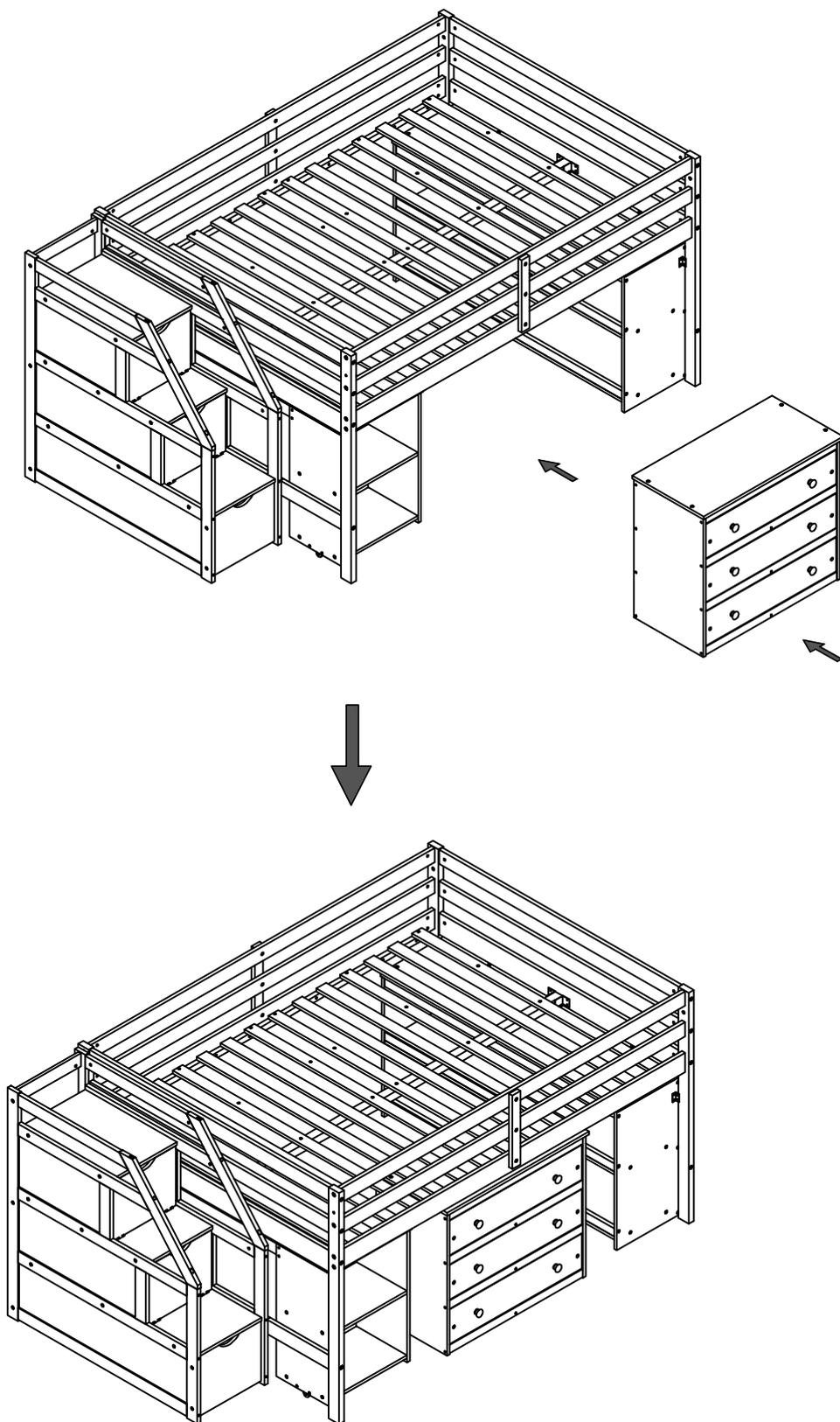
**Make sure to tighten all the screws of the bed.**
